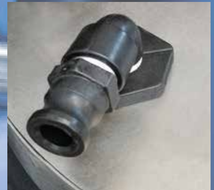
Easy disconnects, feed and returns.
