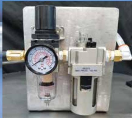
On board regulator and oil fogger
